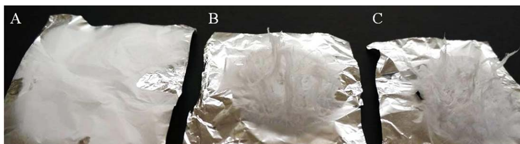
Figure 7. Images of electrospun PEO nanofibers with (A) 0 wt % embedded urea, (B) 20 wt % urea, and (C) 25 wt % urea that demonstrate that there is an increase in the thickness of the three-dimensional web of fibers as the urea content of the polymeric solution is increased. [Color figure can be viewed in the online issue, which is available at wileyonlinelibrary.com .]
